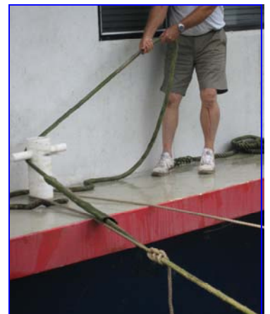
Tightening mooring line using a rolling hitch
